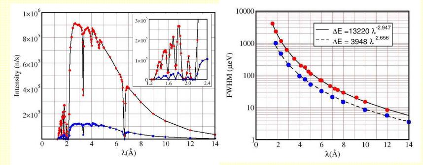
Quantities that can be varied/chosen:Quantities that can be varied/chosen:Chopper period T\*Chopper slot widths WWavelength  $\lambda$ "Speed ratio denominator" m=T<sub>S</sub>/T\* Normally T=3000 µs(T<sub>S</sub> is period at sample)
