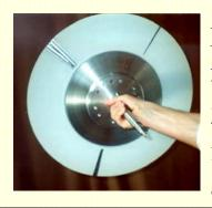
The *pulsing* and *monochromating* choppers are counter-rotating pairs, permitting a choice of pulse widths; they normally run at 20,000 rpm. The *order removal* choppers remove contaminants (also 20,000 rpm). The *frame removal* chopper alleviates the problem of frame overlap; it runs at 20,000/m or 20,000(m-1)/m rpm, where m is a small integer.
